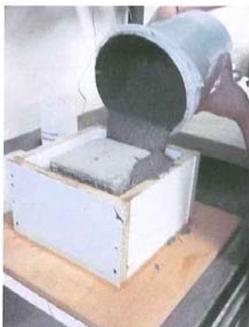
Preparation of the specimen: : casting of REFOR-tec® as a jacket of 30 mm around the concrete prism in the formwork
