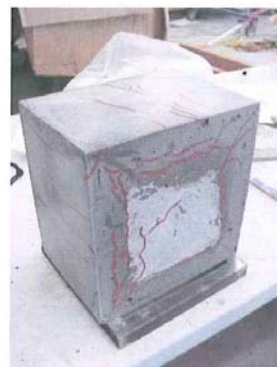
Specimen at end of testing of the shear adhesion
