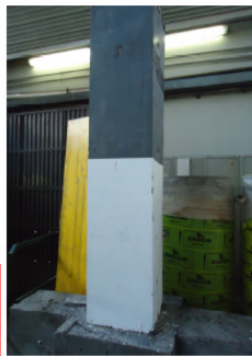
Integral beam after the "hinge" test, with displacement up to 64 mm
