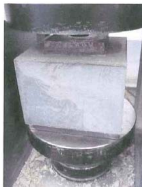
Method of testing : compression on the concrete prism with a metal plate, which is smaller than jacket of REFOR-tec®
